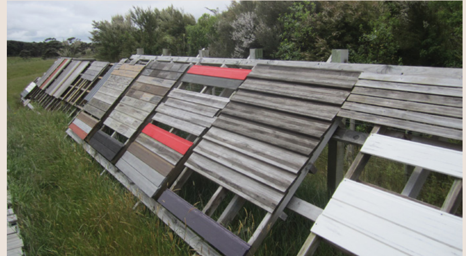
○ Flat panel test racks, Tupare.
