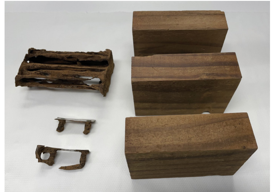
○ Comparative performance of Abodo Vulcan Radiata 230°C untreated (left) vs LOSP Azole and permethrin treated (right), when exposed to Coptotermes acinaciformis termites in AWPC H3 field test, Queensland.
