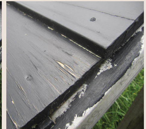
○ MCA treated kiln dried Radiata pine, 3 years exposure.
